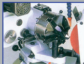
The shoulder of stepped drills may be ground
